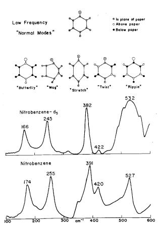
Oscillatory movements associated with the far IR-absorption maxima.
